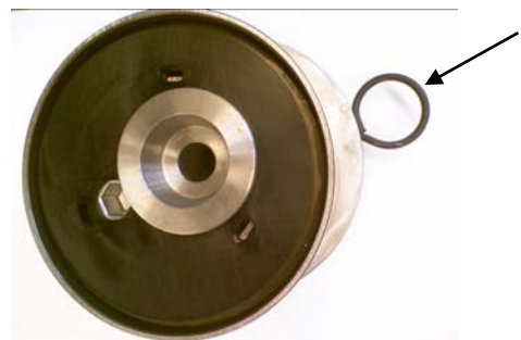
Fig. 2 Pulley design without pin
