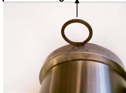
Fig. 3: Variant 2 – withdraw pin after fitting belt
